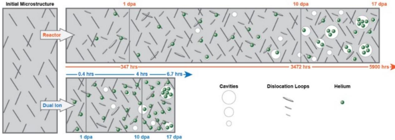
Schematic of the time-dependent helium trapping and release behavior under reactor and ion irradiation conditions
