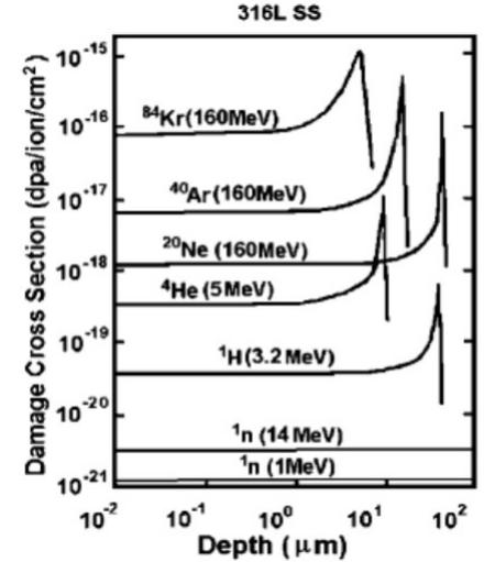
Comparison of damage cross sections for different ion and neutron beams
