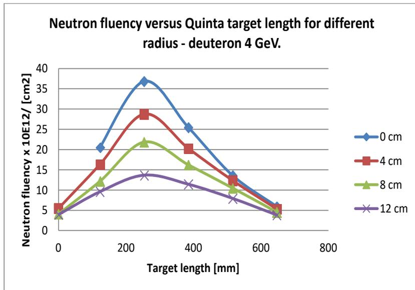
Fig. 4. Neutron fluency distribution versus target length for four different radiuses.
