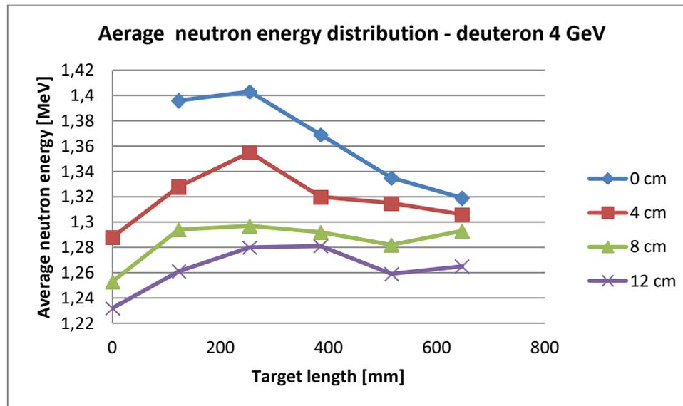
Fig. 2. Axial distribution of estimated average neutron energy for different radiuses.
