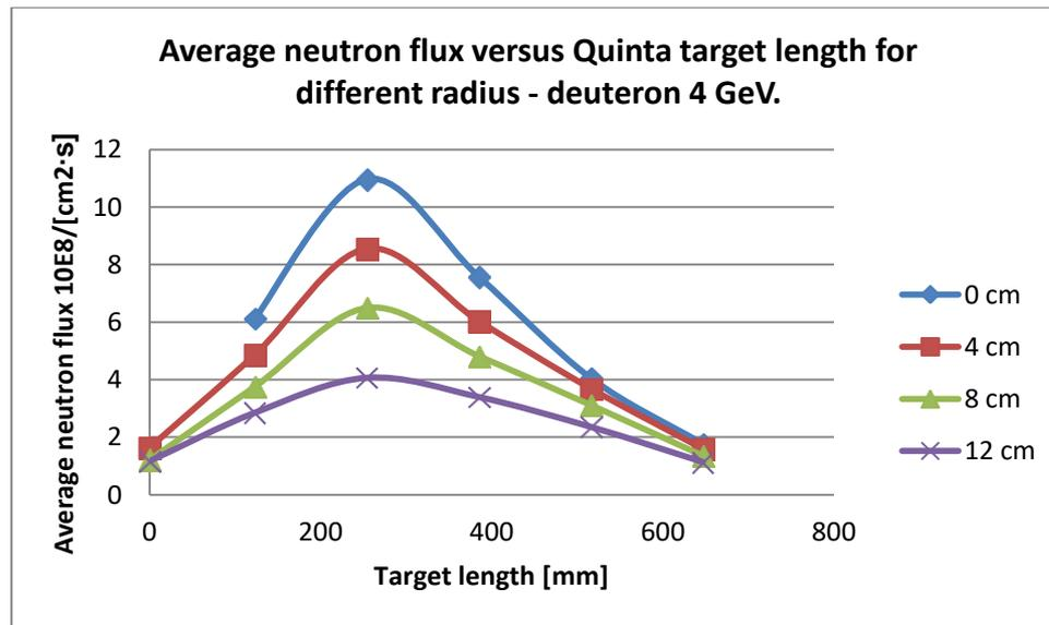
Fig. 3. Average neutron flux distribution versus target length for four different radiuses.
