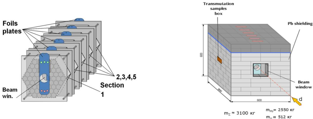
Fig. 1. Schema of Quinta assembly. On the left there is a view on the uranium target with supporting structures and plastics used for sample placement (detector's plates), on the right there is a view on the lead shielding enfolding the target with marked the transmutation samples box (window) for the actinides sample location in the shielding.
