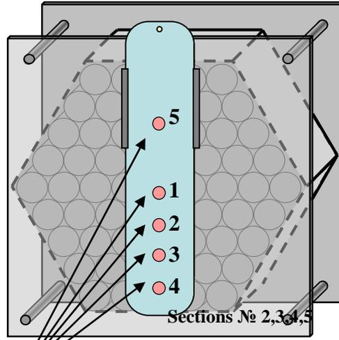
The layout of the uranium foils location on the detector plate. Each plate have 5 positions at the different distances..
