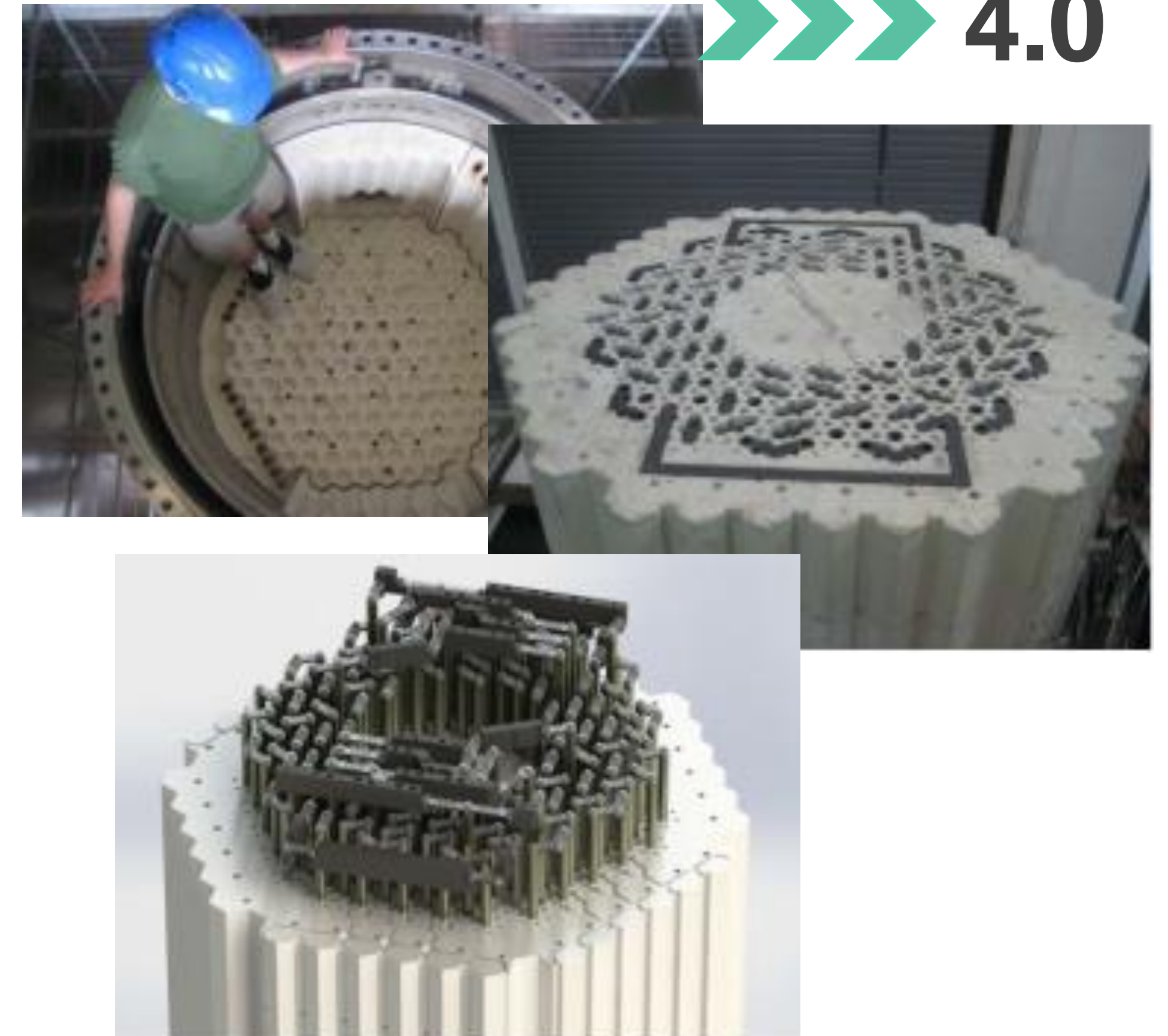
The Oregon State University High Temperature Test Facility (OSU-HTTF): assembly, core and electrical connection of the resistance heater rods.
