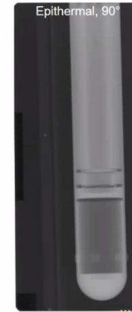
Neutron radiograph of Capsule 1
