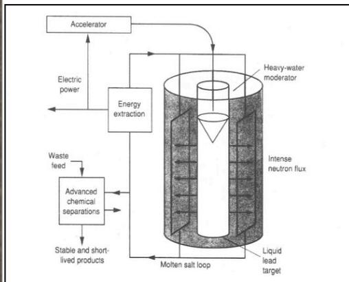
**Rubbia's CERN Fast EA (Energy Amplifier):** The molten lead pool is 30 meters high and 6 meters in diameter. It contains 10000 tons of molten lead.
