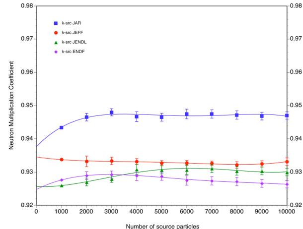
Figure 1: the variation of the multiplication coefficient ( $k_s$ ) in function of the different ND, over the number of simulated protons (ThPu Case).
