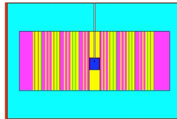
The core consists of a hexagonal lattice immersed in lead and it is composed of 126 fuel assemblies, each loaded with 27 fuel pins. The fuel in the active core region is composed of 85% ThO<sub>2</sub> and 15% <sup>239</sup>PuO<sub>2</sub>. *(The addition of plutonium was necessary to achieve an operational multiplication factor of ~ 0.98 at the beginning of cycle).* The ENDF/B-VI nuclear data library was used
