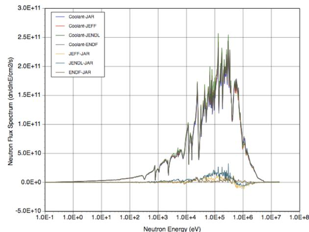
□ Figure 4: Neutron Spectra divergences with ND for the coolant in LEU.
