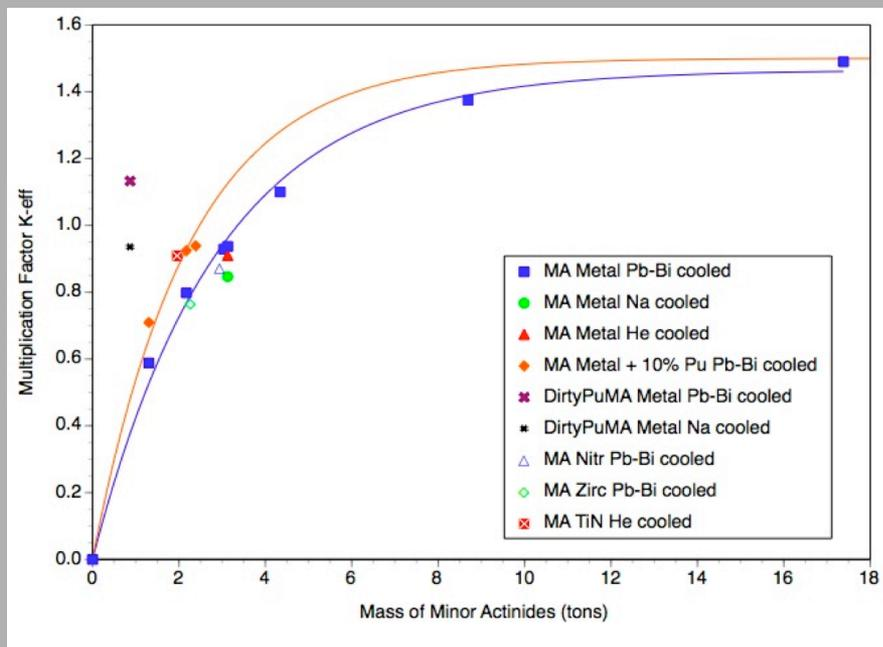
Figure 1: Multiplication coefficient for different fuel mixtures
