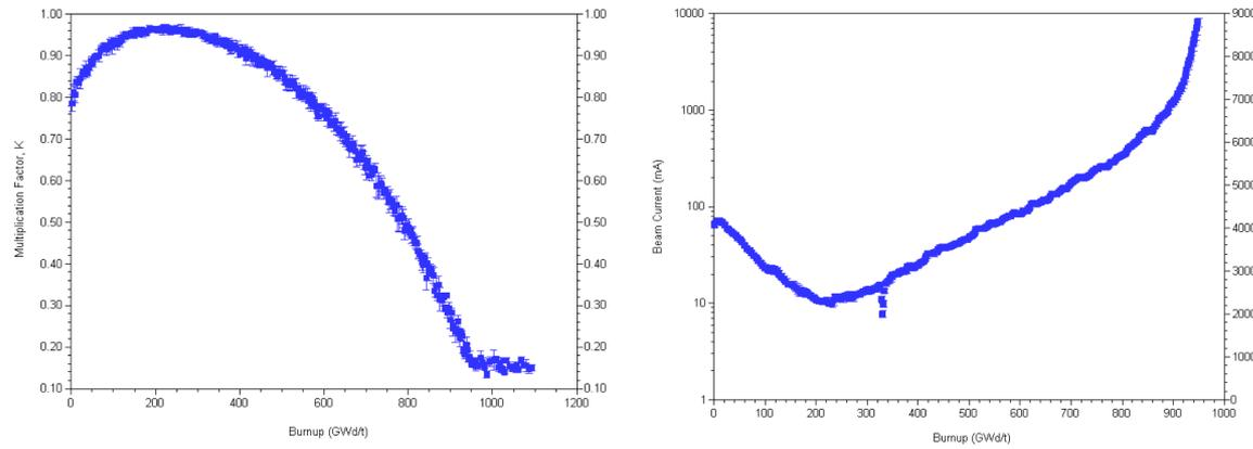
Figure 1: (a) time evolution of  $k$ , and (b) accelerator current
