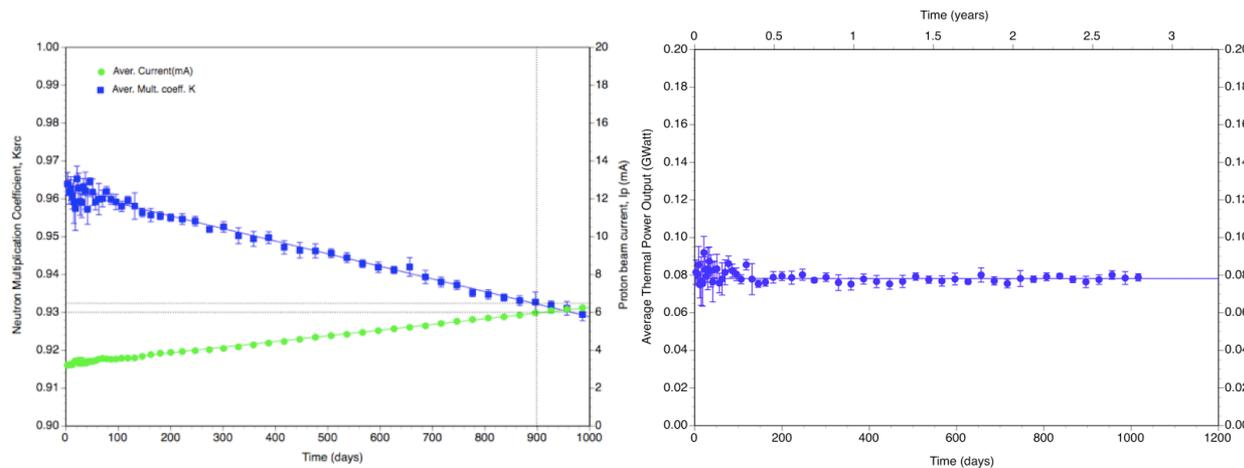
Figure 2: (a) Linear time evolution of the multiplication coeff. and the intensity of the proton beam current of the system over a 900-day burnup cycle; (b) Thermal power of the system. (Initial fluctuations are mainly due to the first days short-lived FF isotopes)
