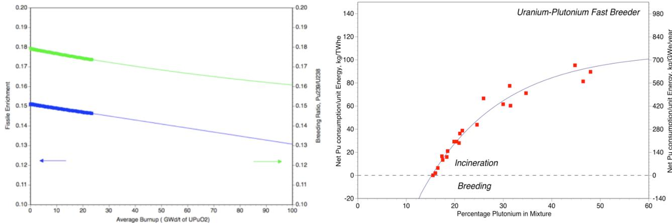
Figure 1: (a) Evolution of fissile enrichment level and the breeding ratio of the system over a 900-day burnup cycle
