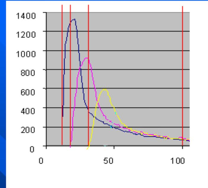
Fig. 2. Cross-sections of the three yttrium (n,xn) reactions – threshold energies:  $E_1 = 11,5$  MeV  $Y^{88}$ ,  $E_2 = 20,8$  MeV  $Y^{87}$ ,  $E_3 = 32,7$  MeV  $Y^{86}$
