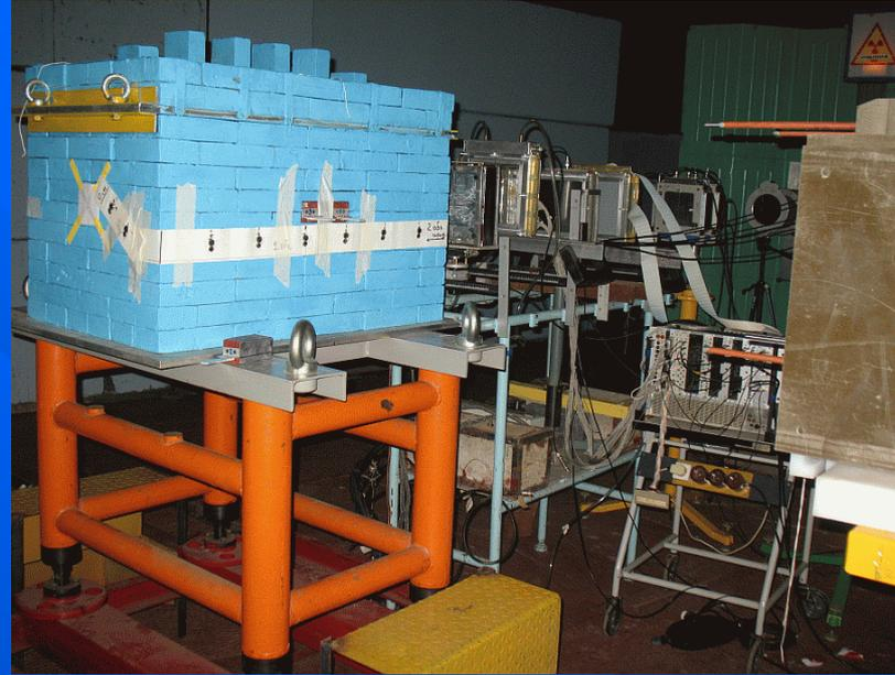
The Quinta sometimes is surrounded by lead bricks 100 mm thick on all six sides of total weight 1780 kg. Shield work as a neutron reflector and as a biological shielding for  $\gamma$ -rays. In the front is a square window 150x150 mm.
