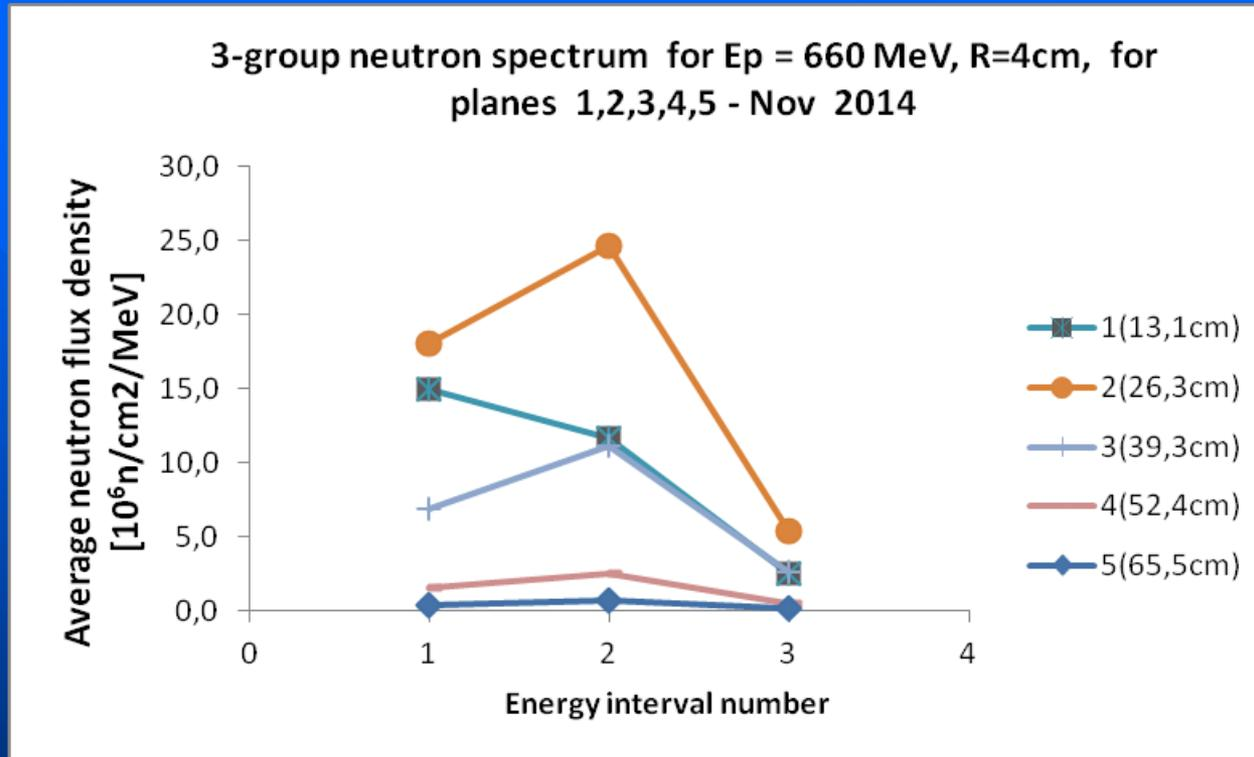
Fig.3. Average neutron flux density versus three different energy range: 1-> (11,5-20,8 MeV), 2-> (20,8-32 MeV), 3-> (32-100MeV) for  $R=4$  cm and five planes (number of successive planes 1,2, 3, 4 and 5) ; proton beam energy 0.66 GeV; Experiment: Nov 2014.
