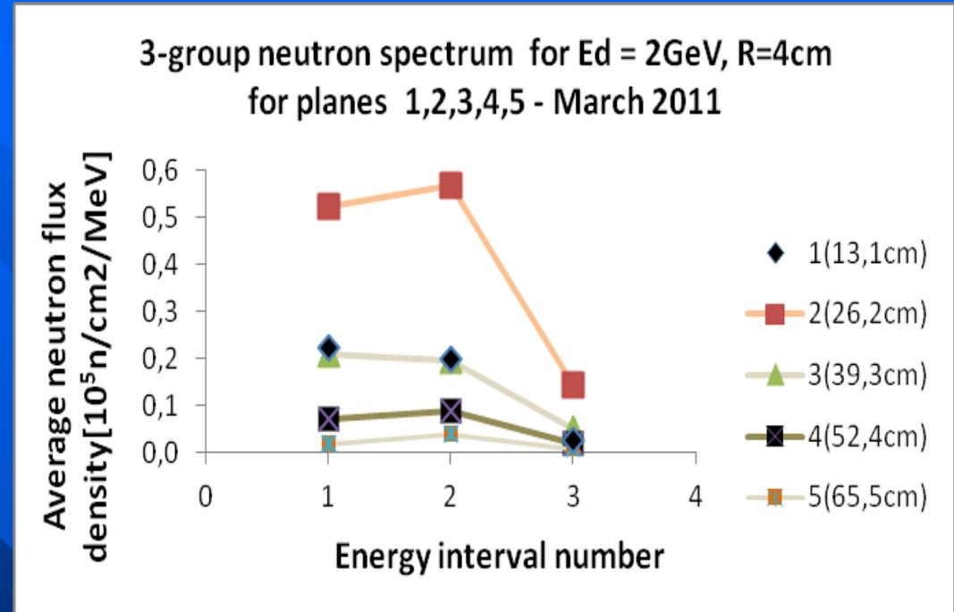
Fig. 4. Average neutron flux density versus three different energy range: 1- (11,5-20,8 MeV), 2- (20,8-32 MeV), 3- (32-100MeV) for R=4 cm and five planes (number of successive planes 1,2, 3, 4 and 5) ; deuteron beam energy 2 GeV; Experiment: III 2011
