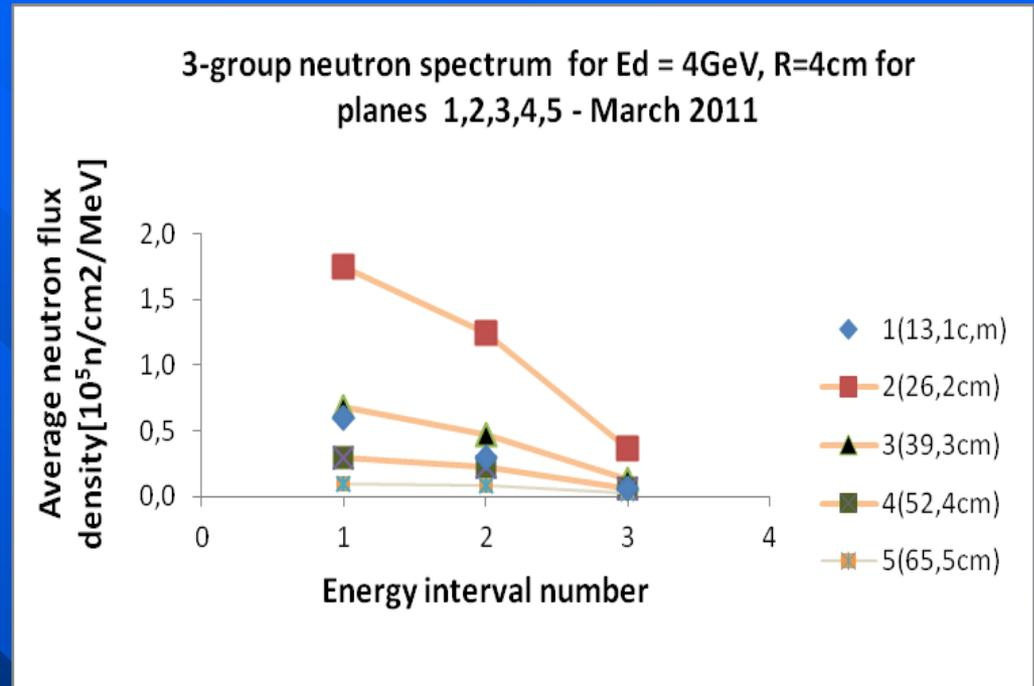
Fig.5. Average neutron flux density versus three different energy range: 1-> (11,5-20,8 MeV), 2-> (20,8-32 MeV), 3-> (32-100MeV) for R=4 cm and five planes (number of successive planes 1,2, 3, 4 and 5) ; deuteron beam energy 4 GeV; Experiment: III 2011
