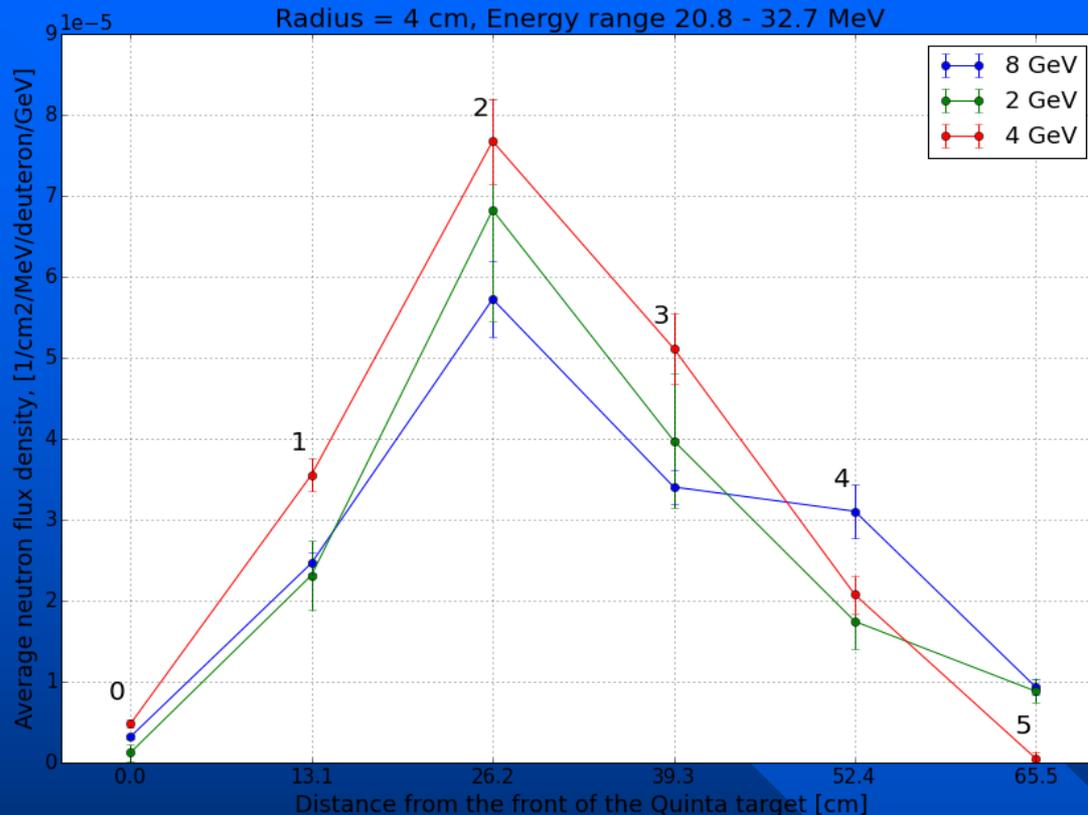
Fig. 3. Average neutron flux density per deuteron and its energy in function of the Quinta target axis at  $R=4$  cm for three deuteron energies (2-top line, 4 middle line, 8-bottom line at position “2”-26.2cm) GeV, in the neutron energy range (20.8 – 32.7 MeV). Errors range  $< 20\%$ .
