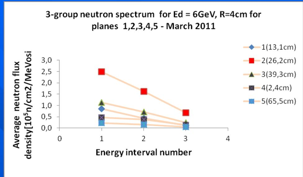
Fig.6. Average neutron flux density versus three different energy range: 1-> (11,5-20,8 MeV), 2-> (20,8-32 MeV), 3-> (32-100MeV) for R=4 cm and five planes (number of successive planes 1,2, 3, 4 and 5) ; deuteron beam energy 6 GeV; Experiment: III 2011
