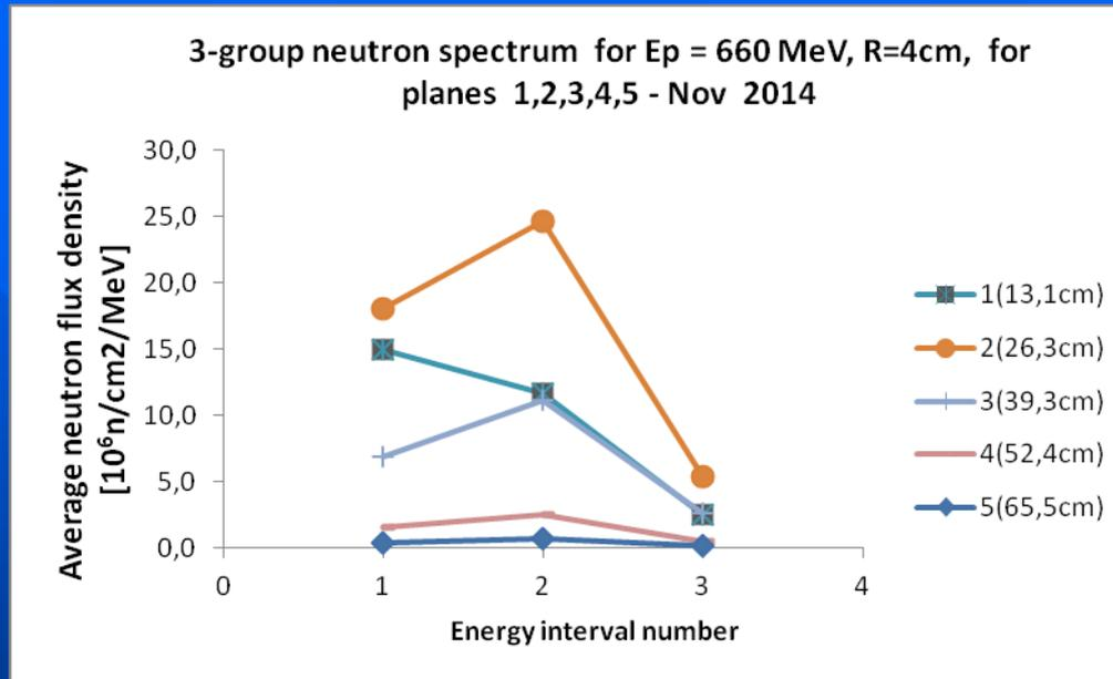
Fig. 1. Average neutron flux density versus three different energy range: 1-> (11,5-20,8 MeV), 2-> (20,8-32 MeV), 3-> (32-100MeV) for  $R=4$  cm and five planes (number of successive planes 1,2, 3, 4 and 5) ; proton beam energy 0.66 GeV; Experiment: Nov 2014.
