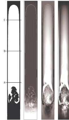
DNS simulation of slug flow
