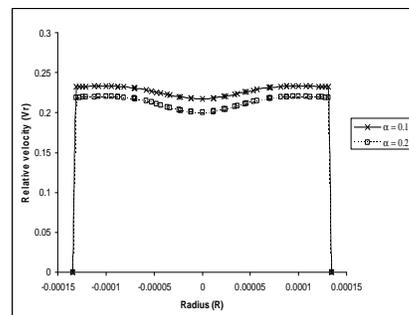
Calculated relative gas-to-liquid relative velocity
