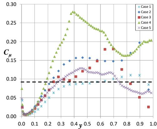
DNS-predicted lateral distribution of  $C_\mu$  (Bolotnov & Podowski, 2012). Case-1 corresponds to single-phase flow, and Case-2 through Case-5 represent two-phase flows for different bubble sizes and gas/to-liquid density ratios
