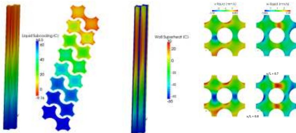
Three-dimensional distributions of temperature, void fraction and liquid velocity along and between fuel elements in a four-channel section of reactor fuel assembly [Shaver et al., 2015]
