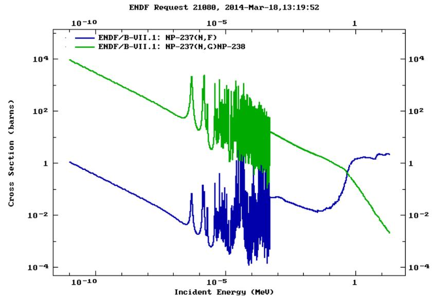
Fig. 1. Cross-sections of Np-237(n,g)Np-238 and Np-237(n,f) reactions.
