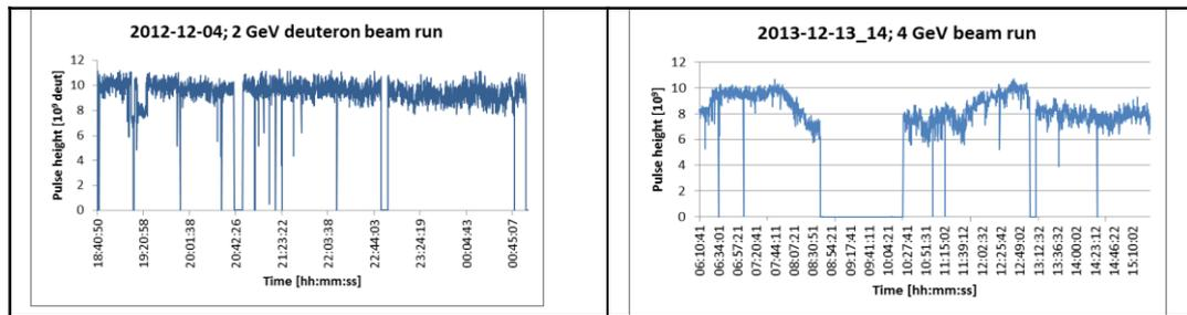
Fig. 3. Distribution of deuteron pulses during the irradiation period as measured with an ionisation chamber.
